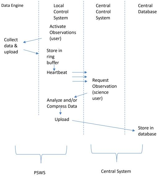
Figure 2. Use Case 1. Request/Response process model.
